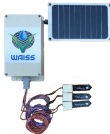
Figure 1. Water Advisory for Irrigation Scheduling System (WAISS) field unit with capacitance-type soil moisture sensors, transmitting data logger, and solar panel.
